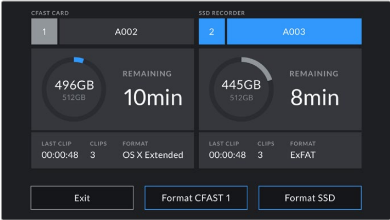
When an SSD is inserted into URSA Mini Recorder, your camera's storage manager will display 'SSD Recorder' over storage slot 2.
