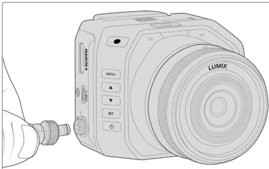
Connect power to your camera's power input using the supplied cable
