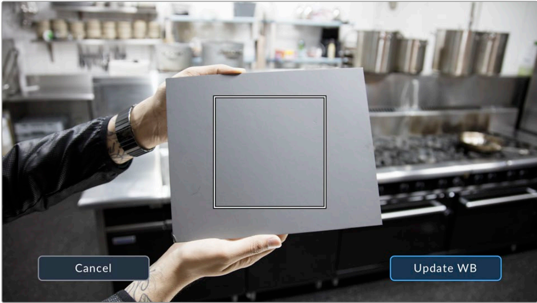
Use this with a white or neutral gray surface to automatically set a neutral white balance
